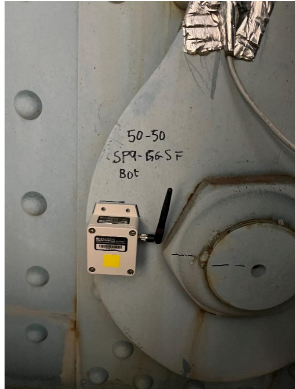
Wireless medium resolution tiltmeter (inclinometer) SenSpot™ at a machinery equipment
