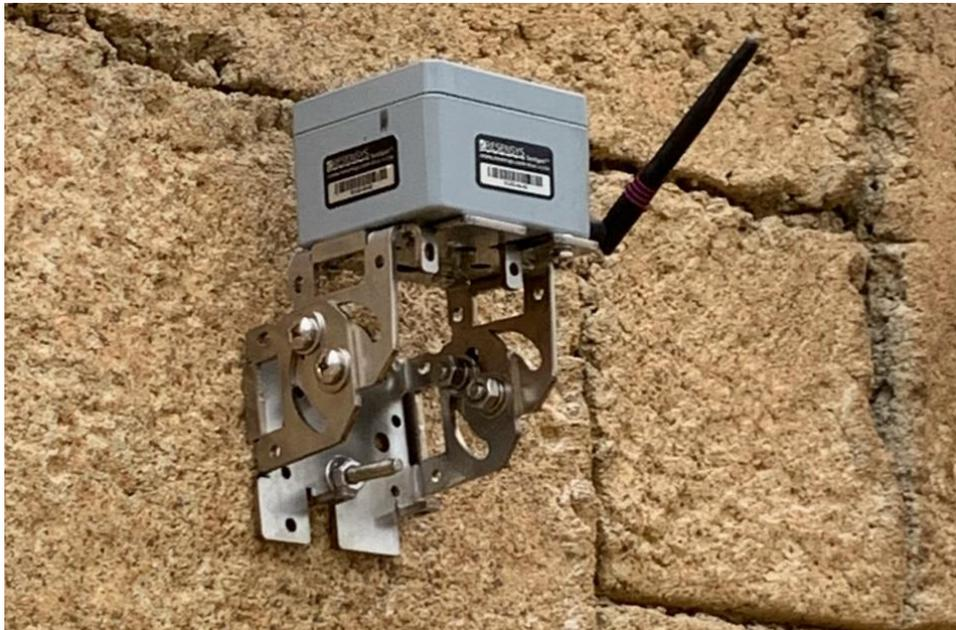
Figure 4: A Resensys 2DHRT SenSpot™ installed on a retaining wall
