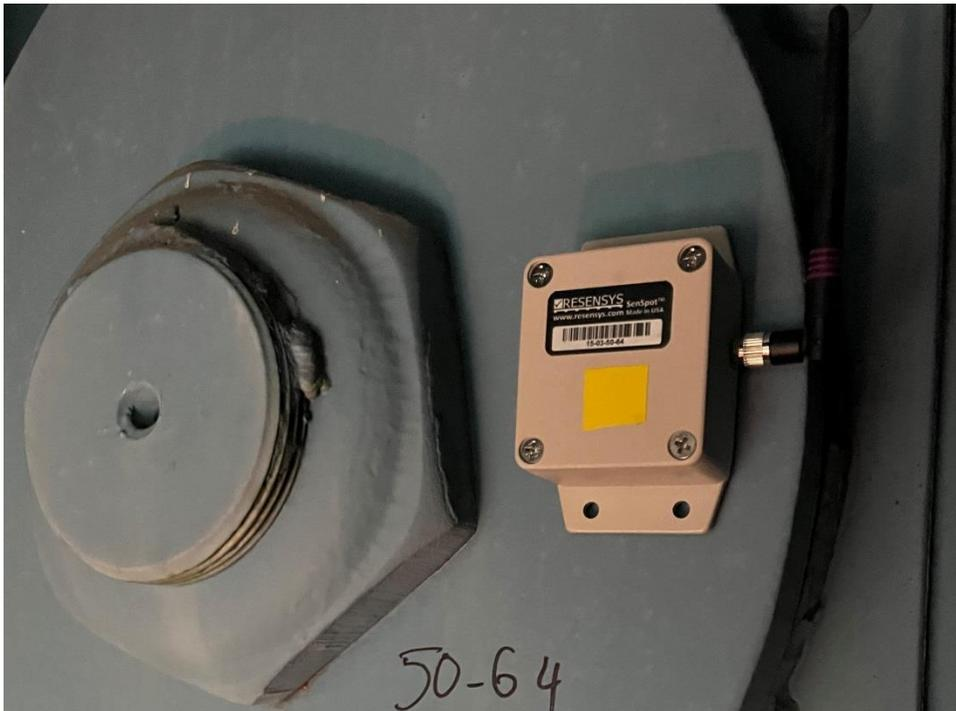
Figure 4: A Resensys 2DMRT SenSpot™ installed on a bridge bearing
