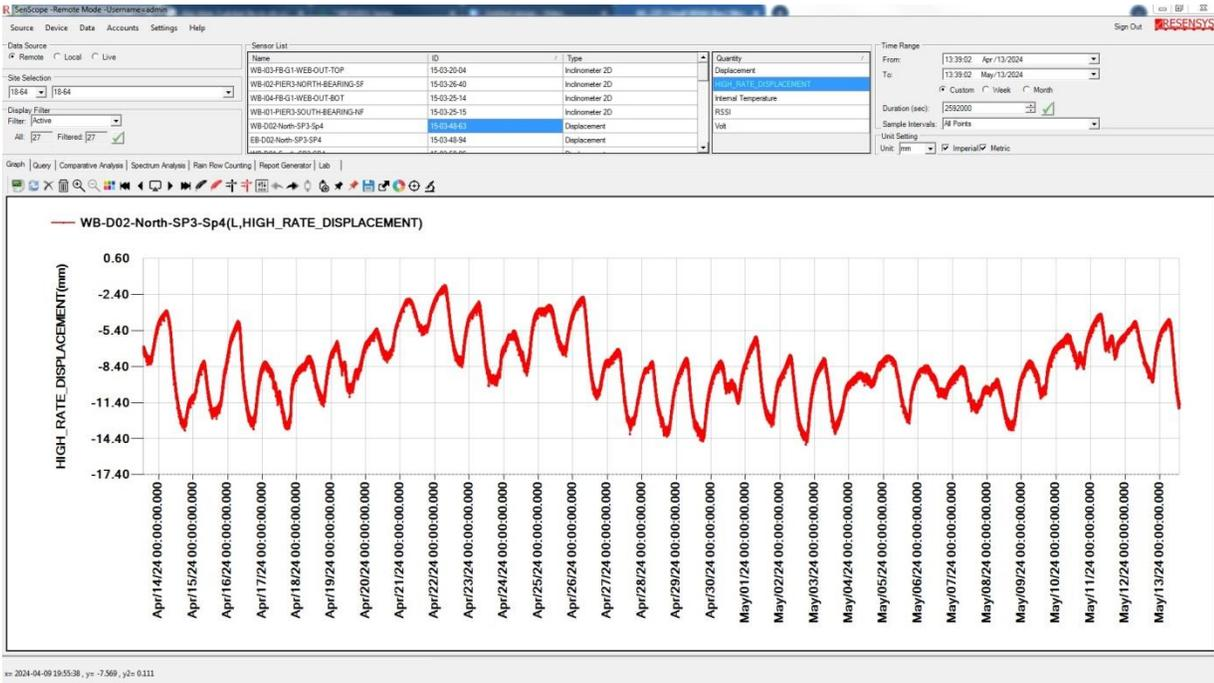
Figure 3: One month of High-rate displacement measurements of an installed SenSpot™
