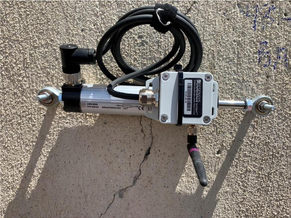
Figure 4: Installed displacement SenSpot™ on a concrete tower for monitoring crack width development
