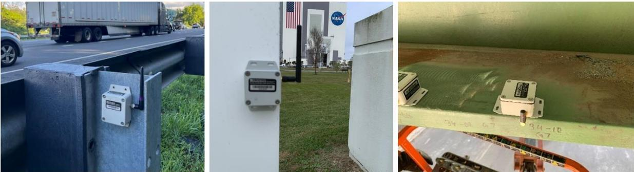
Figure 4: Resensys High Performance Accelerometer (HPA) SenSpot™ sensors installed on structures
