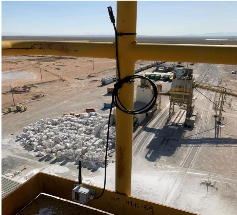
Figure 3: A Resensys wireless Humidity-Temperature SenSpot™ installed on a building inside a mining facility
