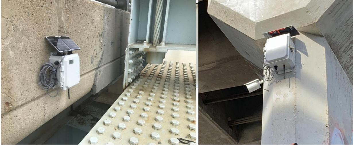
Figure 4: Installed SeniMax™ (left) and SeniMax with camera (right)
